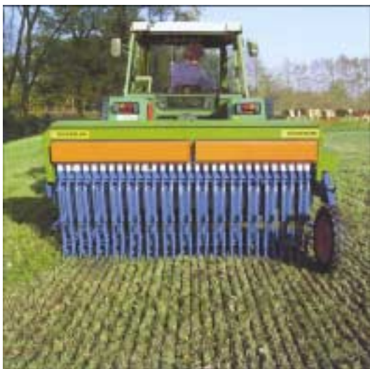
Picture 5. Sowing the seed directly in the existing sward
