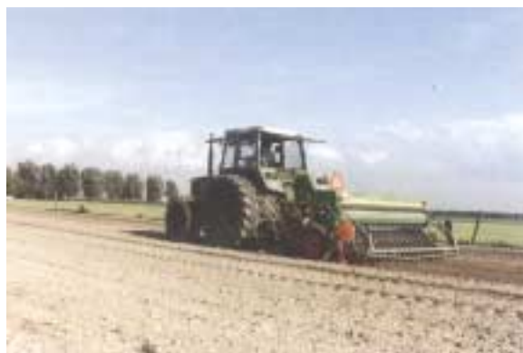
Picture 4. Seedbed preparation and sowing executed in one operation
