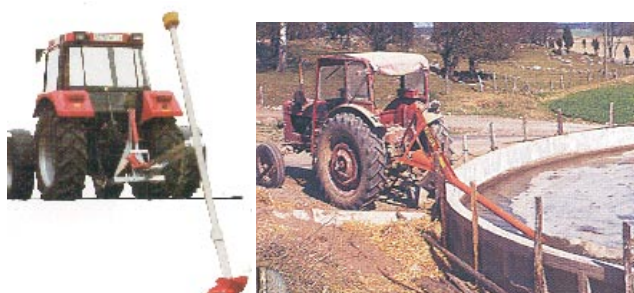
Figure 3. Different kinds of tractor-type mixers for slurry mixing.
